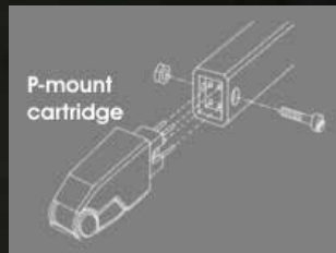
P-mount cartridge mounted on P-mount tonearm (screw and nut are supplied with all models).
